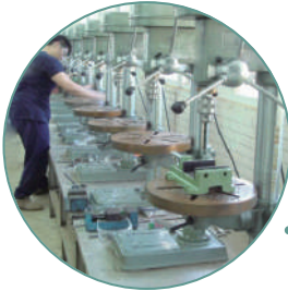
A. Drilling Machine
